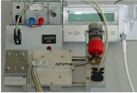
Figure 1 Cyclic fatigue dynamic testing device with mobile platform for simulation of the clinical use of the instruments.
